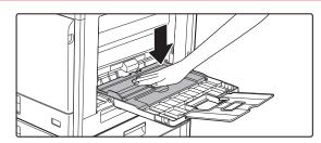
Push the centre of the pressure plate down until it locks into place.
